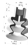
Bellows Suction Cup 2.5 folds Series 8B, Ø 40 mm Product reference: 8B 40-- F14
