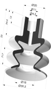
Bellows Suction Cup 2.5 folds Series 8B, Ø 40 mm Product reference: 8B 40-- A
