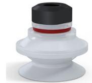
Variant reference: 91 31SLT 18D-2-F • Color: Translucent • CE food certified • Matter: Silicone • Shore Hardness: SH60
